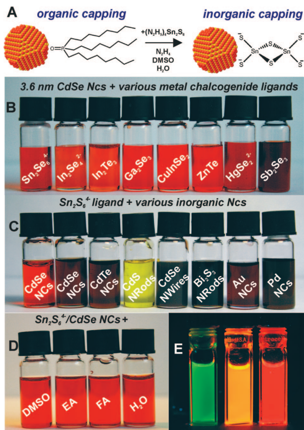
Figure 15. (A) A sketch of a generic exchange of original organic ligands by metal chalcogenide complexes: the original organic ligands (TOPO) at the surface of CdSe NC are replaced by Sn 2 S 6 4- Zintl ions. (B) Stable colloidal solutions of 3.6 nm CdSe NCs capped with various metal chalcogenide complexes in hydrazine. (C) From left to right: stable colloidal solutions obtained by combining (N 2 H 5 ) 4 Sn 2 S 6 with 3.6 and 5.8 nm CdSe NCs, 9 nm CdTe NCs, 5 × 60 nm CdS nanorods (NRods), CdSe nanowires (NWires), ~25 nm wide, 2–5 μm long, 6 × 25 nm Bi 2 S 3 NRods, 5 nm Au NCs, and 3 nm Pd NCs. (D) From left to right: CdSe/Sn 2 S 6 4- NCs dispersed in dimethylsulfoxide, ethanolamine, formamide, and water. (E) Photograph of NC photoluminescence excited by a UV lamp. From left to right: 2.9 nm CdSe/Sn 2 S 6 4- NCs in EA (green emission, quantum yield QY ≈ 2%), 3.6 nm CdSe/Sn 2 S 6 4- in DMSO (yellow emission, QY ≈ 3%), and Sn 2 S 6 4- -capped CdSe/CdS core-shell NRods in hydrazine (red emission, QY = 10%). Reprinted with permission from ref 273. Copyright 2009 American Association for Advancement of Science.
