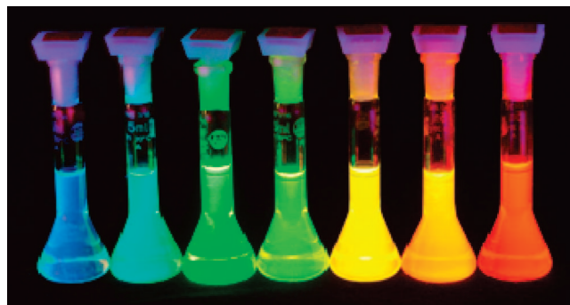
Figure 3. Size-dependent change of the emission color for colloidal solutions of CdSe/ZnS core–shell nanocrystals. The particles with the smallest (~1.7 nm) CdSe core emit blue; the particles with the largest (~5 nm) core emit red. Reprinted with permission from reference 95. Copyright 2002 Wiley.
